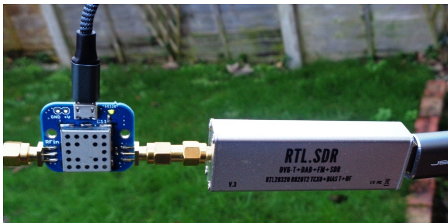
Figure 6: The HI line pre-amplifier and RTL-SDR Blog V3 USB Receiver.
