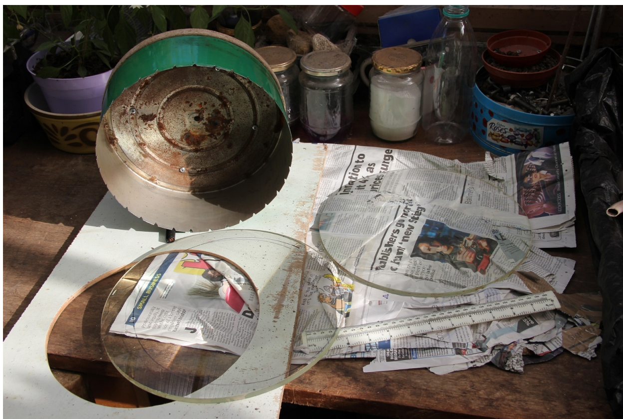
Figure 1: Two 12 inch diameter lenses and the 26cm diameter metal cutter
