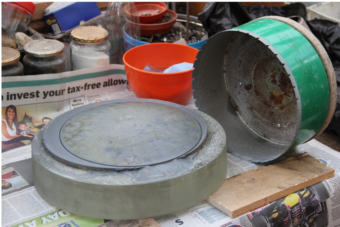
Figure 2: The completed cut on the first prism blank
