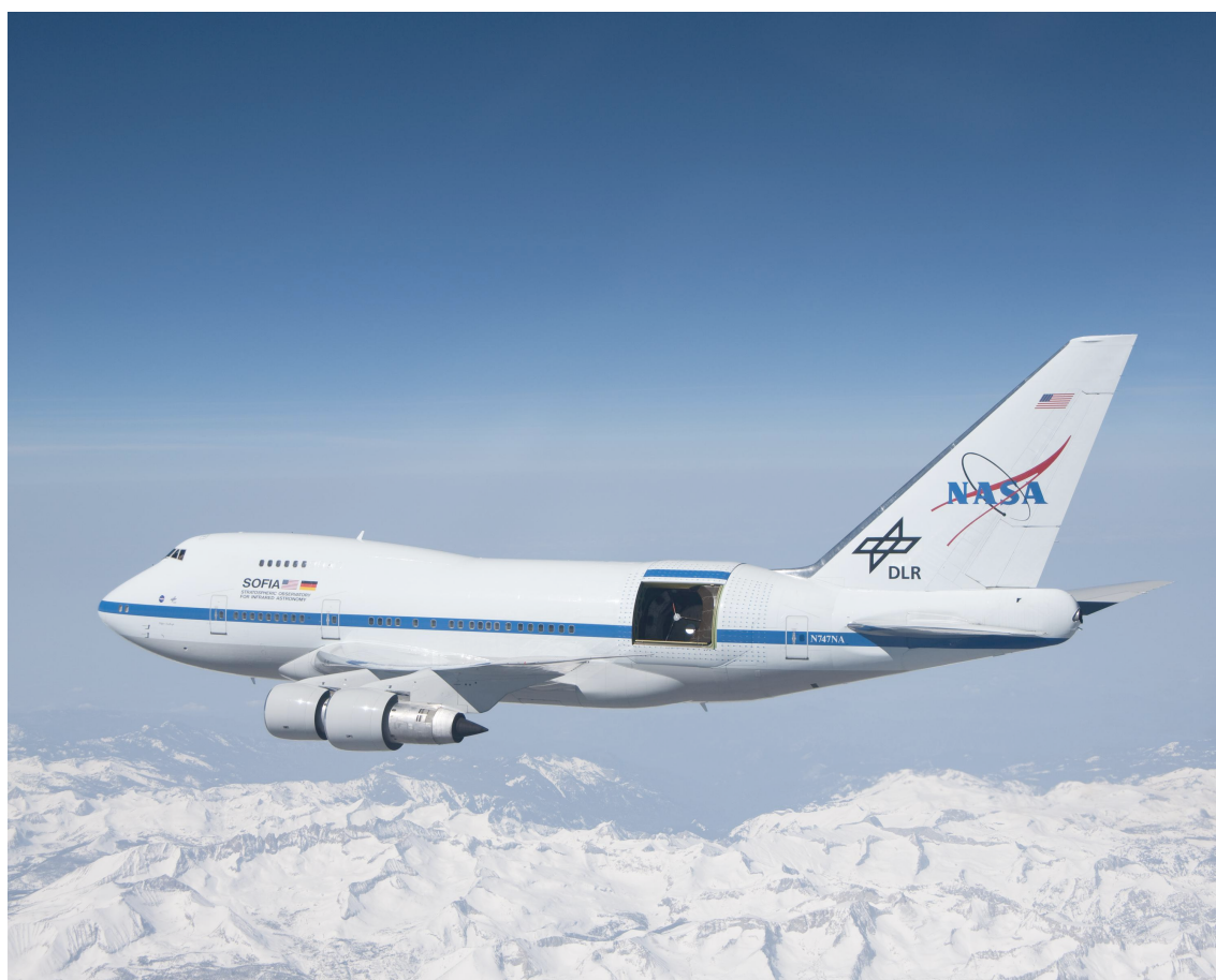
SOFIA soars over the snow-covered Sierra Nevada mountains with its telescope door open during a test flight. SOFIA is a modified Boeing 747SP aircraft.
