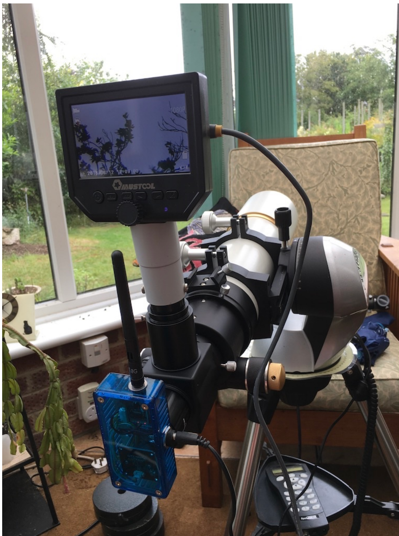
Test set-up with both cameras on the 500mm refractor using a flip mirror, targeted on a distant (~150m) beech tree.
