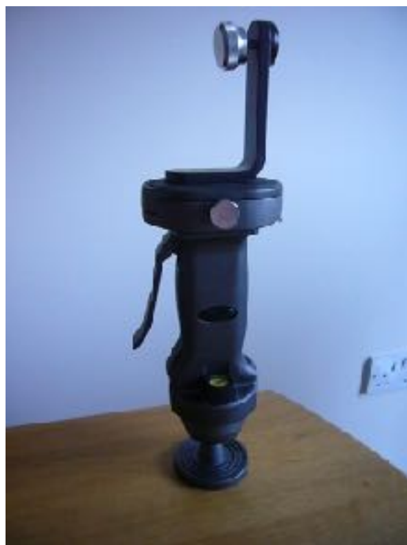
Neewer head and Opticron "L" bracket put together. The head has a ball and socket joint at the base, which is normally locked, but becomes free to move when the trigger lever is pulled.
