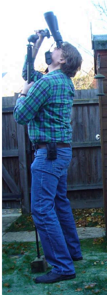
Resting the monopod on a piece of scrap 4"x4" fencepost will help taller people that use this setup at or near the zenith.
