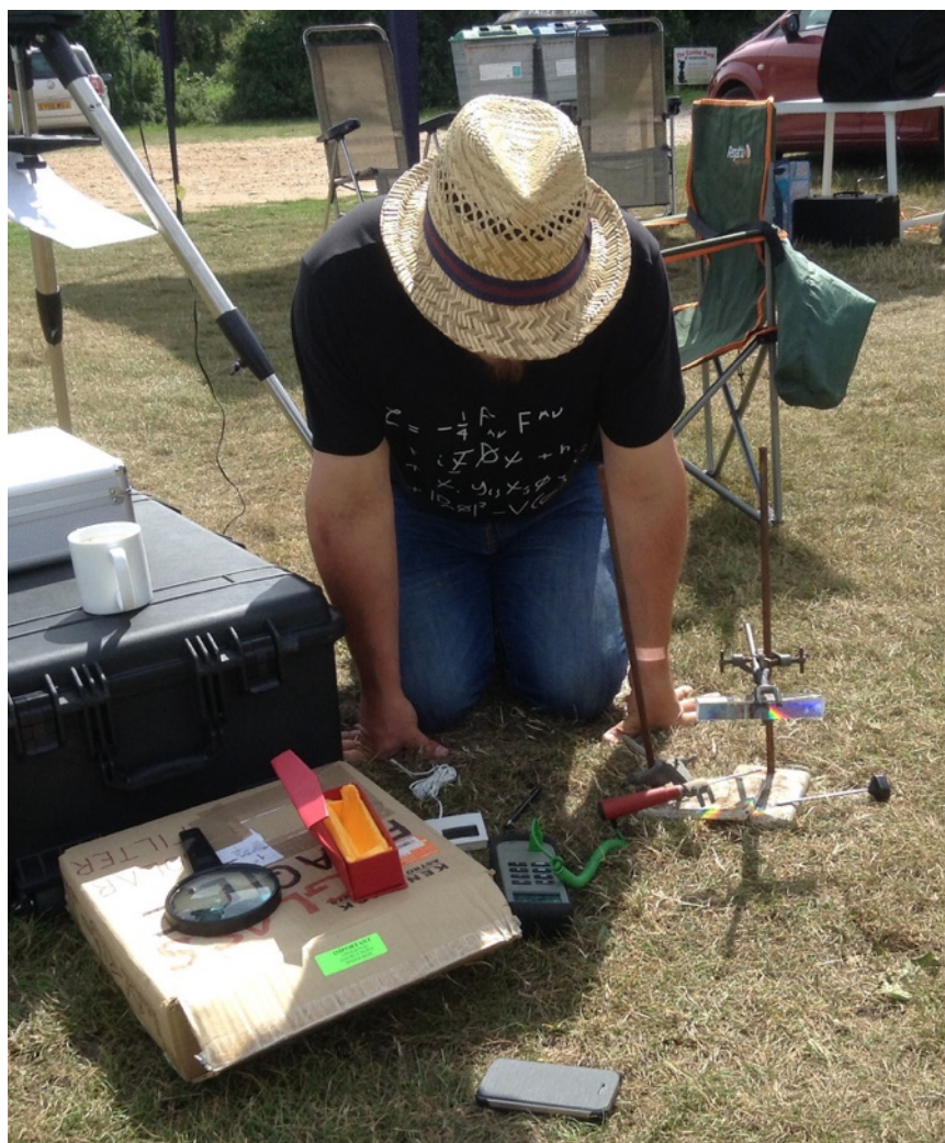
Kevin Fulcher repeating Herschel's experiment, measuring the temperature beyond the red.
