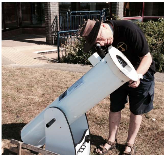
MartinRH finds Sol with homemade finder (off-cut of square drainpipe with 1.5mm pin-hole)
