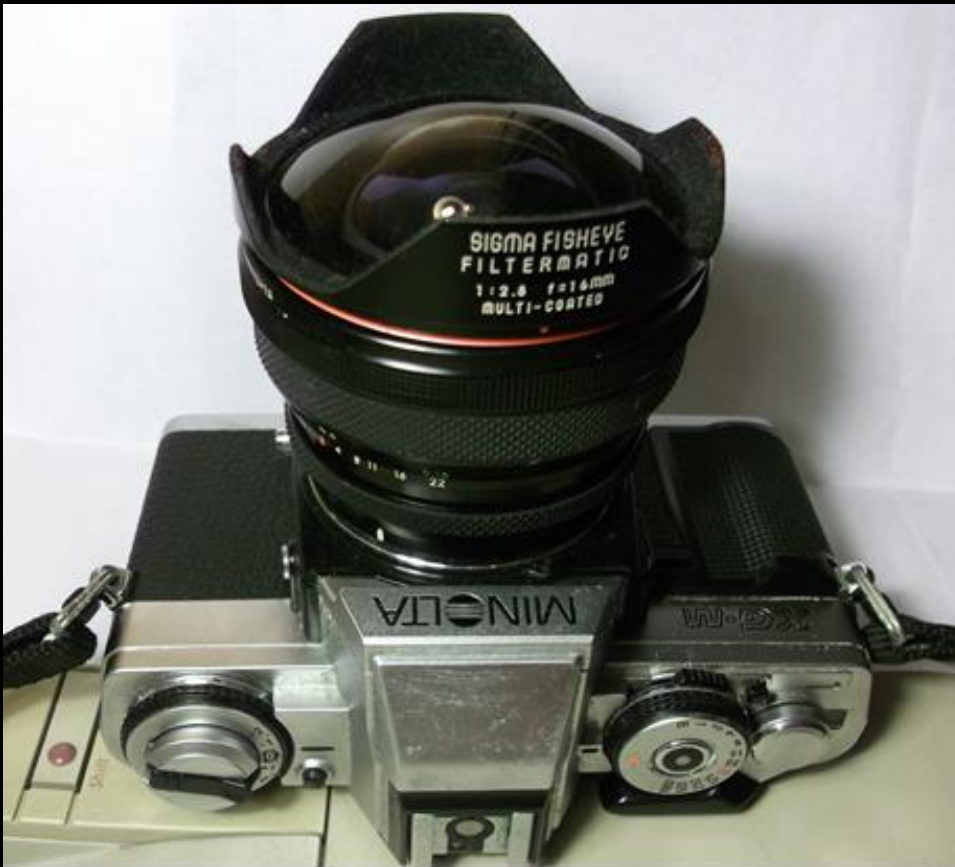
16mm, F2.8 fisheye lens, coupled to a motor-driven, Minolta 35 mm camera.
