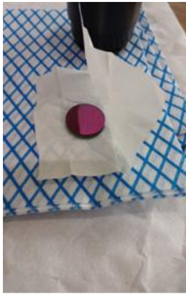
Replacement BelOptik ITF filter before installation.
