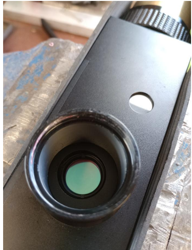
Exposed ITF filter at the base of the eyepiece tube.
