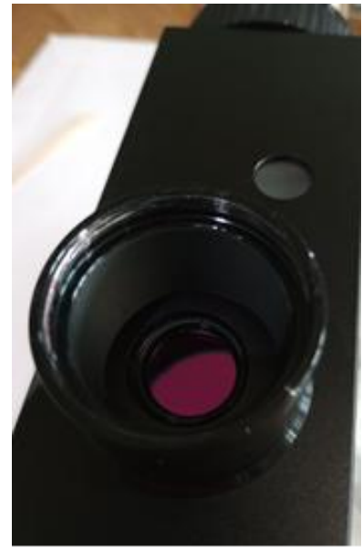
BelOptik ITF filter after installation.
