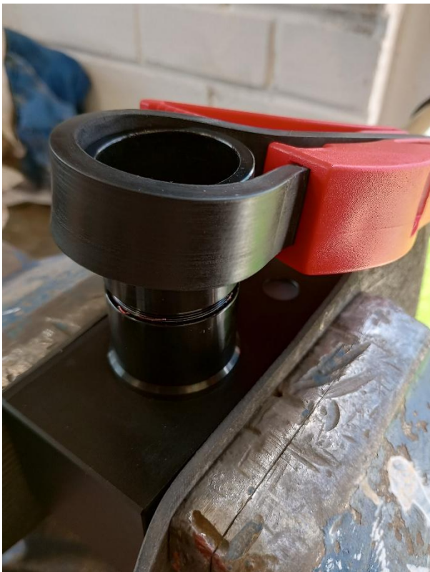
PST body securely clamped in the vice with a strap wrench applied.
