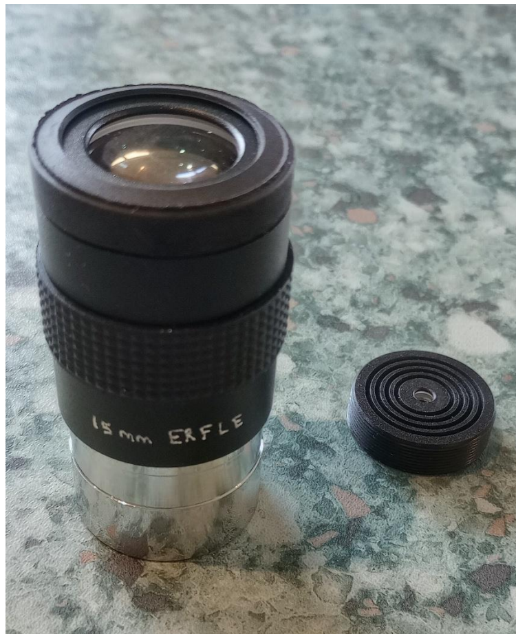
Resulting eyepiece (LHS) with original Smyth lens assembly (RHS).
