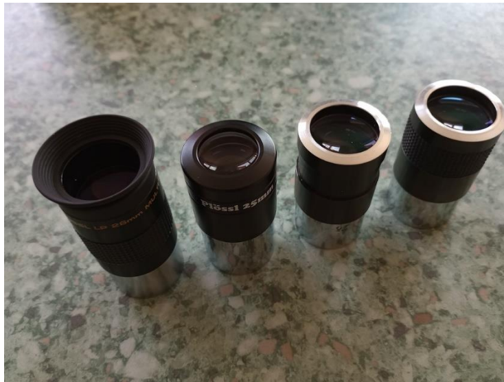
Full Plössl Line-up L-R: original Meade 26mm, Star 25mm, modified Meade 26mm (x2)
