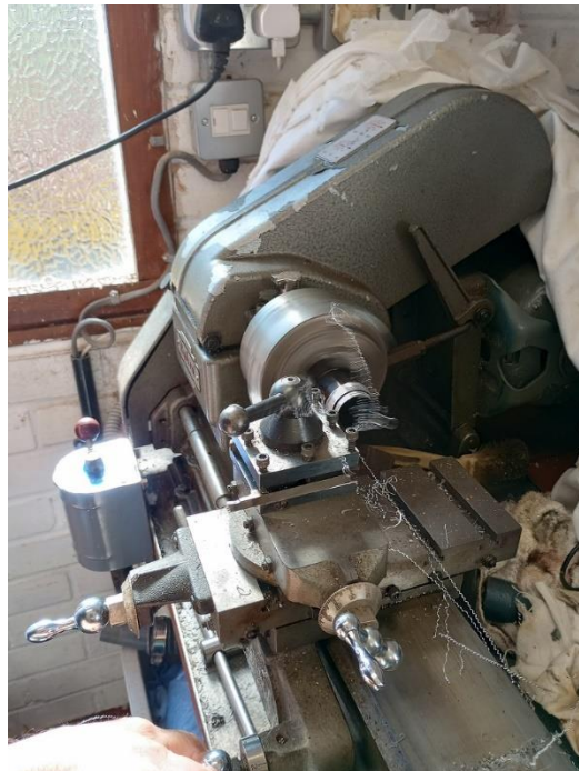
Lathe treatment removing 13mm from the top of the barrel
