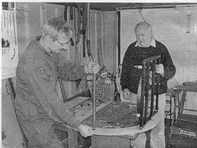
Figure 3 – The mirror cell is now securely bolted to the lower side bearing using three carriage bolts, which hold it firmly in place. Martin is attaching an additional tubular bracing strut to enhance the structural integrity of the entire mirror support system once assembled.
