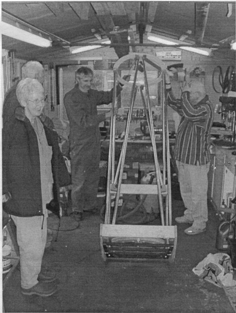
Figure 9 – A cause for celebration!! Truss poles have been inserted into the wooden clamps in the primary mirror system, and secondary ring and spider attached for the first time! This was an incredible and memorable occasion after all the hard work that went into the design and construction. The scope was assembled within 10 minutes. [One key component awaiting final construction and not shown in the photo is the base providing azimuth and elevation movement].
