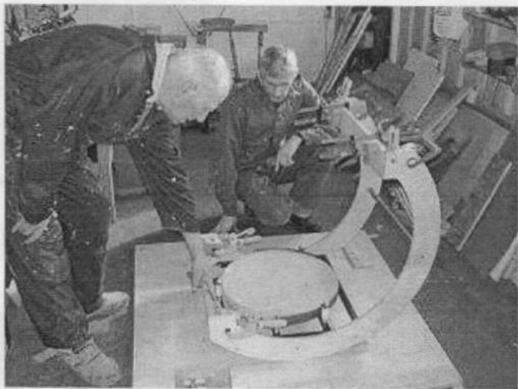
Figure 7 – The mirror cell has been securely bolted to the side bearings using carriage bolts and the metal support-bracing strut has also been fitted. In this photo, two wooden “end battens” and eight wooden Serrurier truss pole clamps holding the
