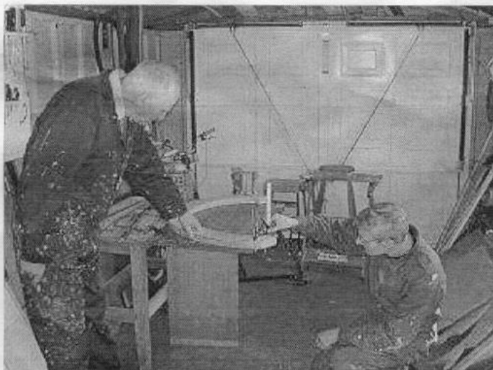
Figure 1 – Checking correct orientation of side bearings and holes correctly marked prior to drilling.
