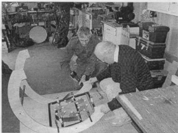
Figure 6 – The upper side bearing has been securely clamped in place and Martin is starting to drill the two remaining holes. The drill passes all the way through!
